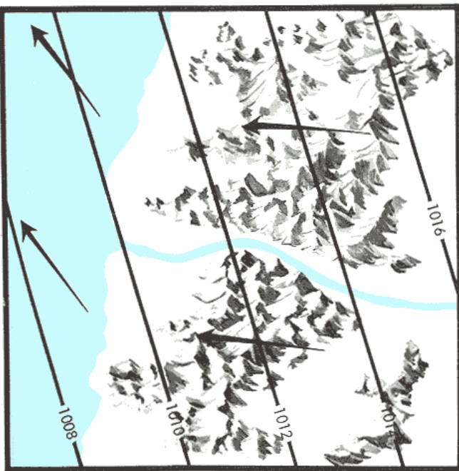
Over rough topography, large frictional effects may cause surface winds to blow almost directly across the isobars from high to low pressure. Where friction is less, such as over water, surface wind directions have only a small angle across the isobars.
