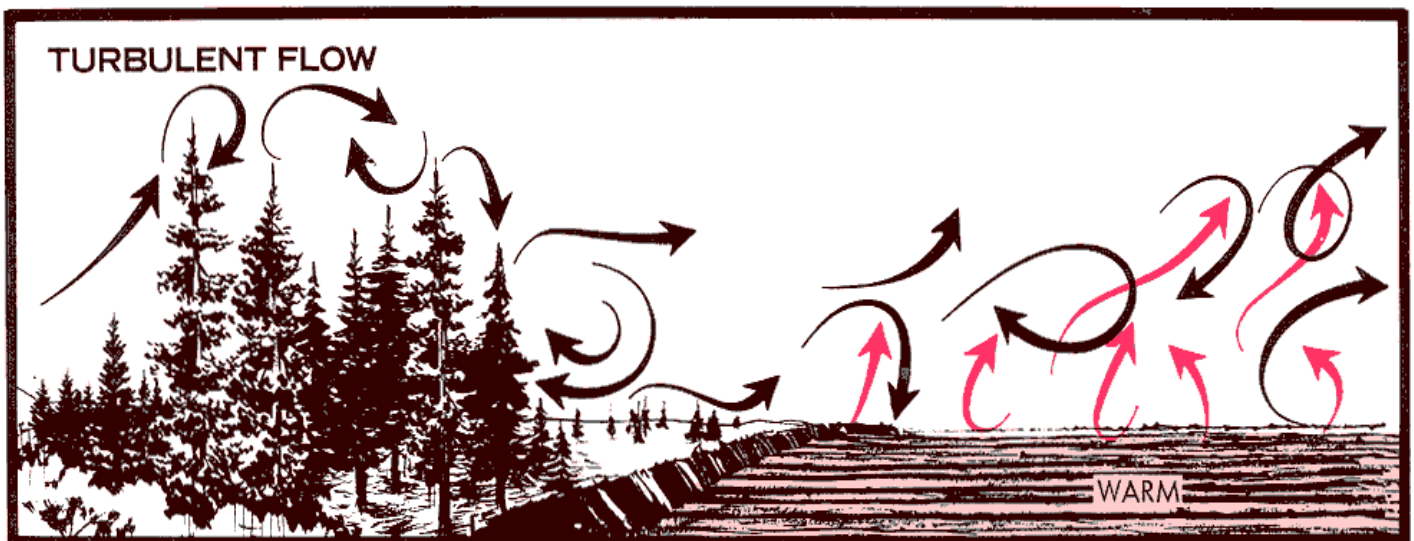
Roughness creates mechanical turbulence, while surface heating causes thermal turbulence in the airflow.
