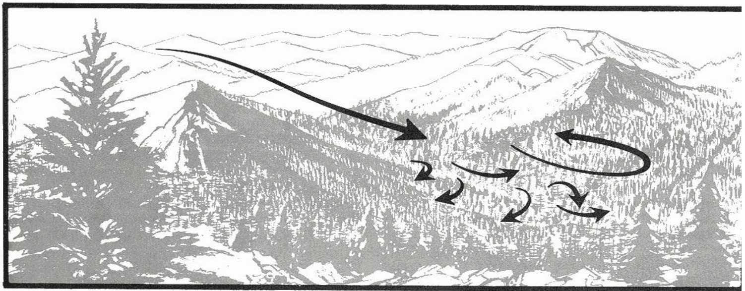
Ridgetop saddles and mountain passes form important channels for general wind flow. The flow converges and the wind speed increases in the passes. Horizontal and vertical form on the lee side of saddles.
